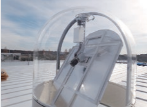
Automatic GPS-based sun tracking system installed above open ceilings
