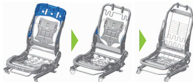
Evolution of the functional parts (blue areas) of the frame
