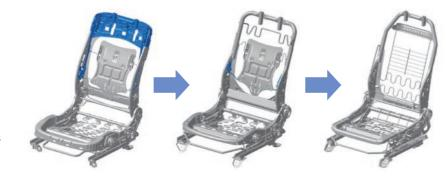
1) Lumbar support: Cushion support that protects the driver's lower back and reduces fatique 2) TS TECH internal comparison
