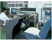
Analyzing ride comfort using body pressure distribution measurement
